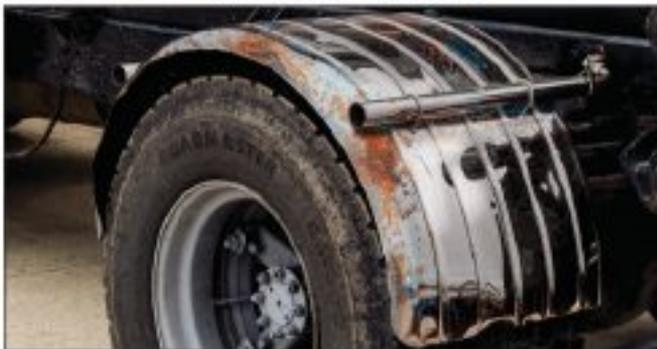
Typical dented, cracked, and rusted metal fenders
