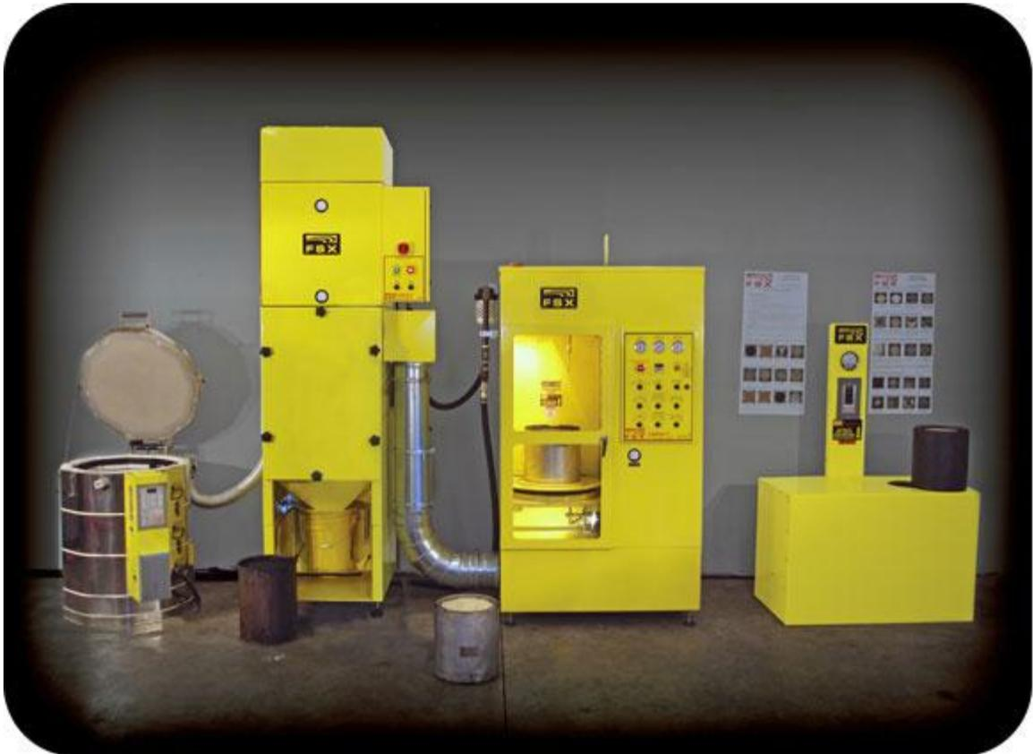
Cleans using Air Knife Scanning technology on both ends of the filter.
